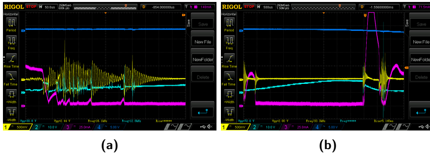
Figure 4.30: The ringings in the receiver antenna when the loop antenna was placed at a 45 degree angle with the rail and the current was 80 A in left picture and 40 A in right picture
