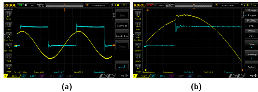
Figure 4.13: A none perfect filtering of the square wave to sine wave in the sending antenna. The blue curve is the driving square wave signal. The yellow curve is the field out from the antenna measured with a magnetic-field probe
