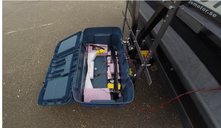
Figure 4.19: The sending circuit mounted on the car
