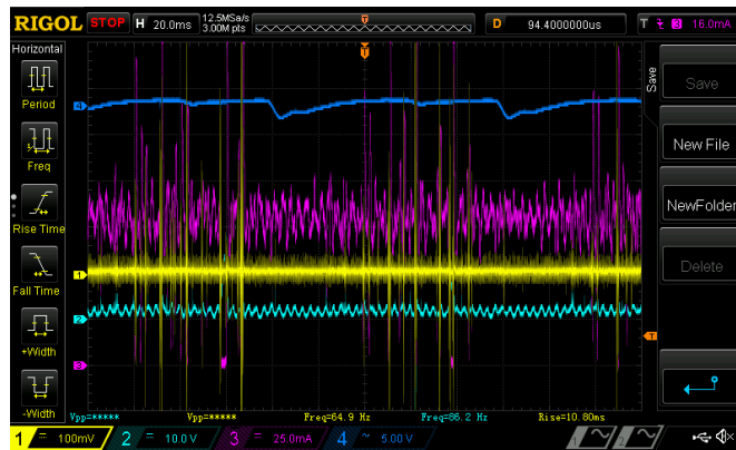
Figure 4.28: The signals that were measured on the oscilloscope. Yellow is the voltage over the receiver antenna located in between the rails, turquoise and magenta are the voltage and the current through the circular tracks and blue is a signal indicating the rotation speed of the sleigh.
