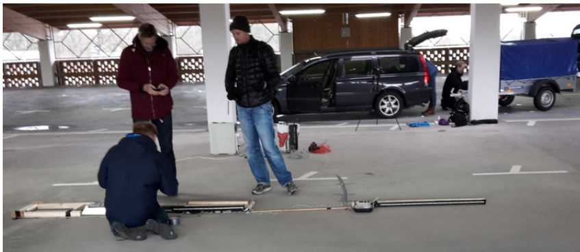
Figure 4.35: The final test setup is being arranged. The car is going to drive over the mock-up from the left in the picture and the LED strips can be seen pointing towards the camera of this picture as the white stripe on the black tape on the mock-up
