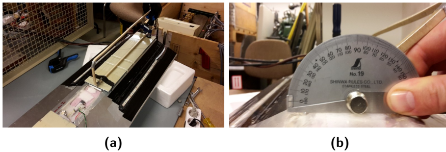
Figure 4.27: On the rail of the prototype there is a loop antenna simulating a pickup. a) In this particular position the pickup is perfectly centered above the rail. b) The pickup has a 45 degrees angle with the rail
