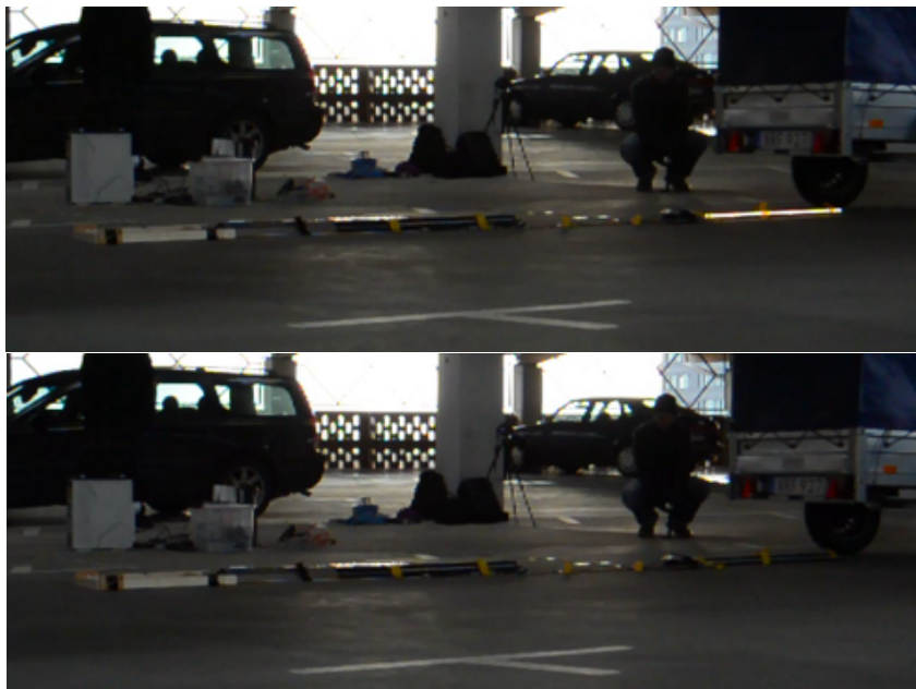
Figure 4.39: The timing of the second rail-computer (Arduino) turning off the second rail segment represented by the LED strip behind the trailer.
