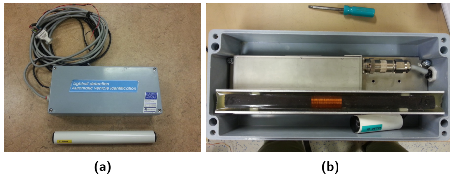
Figure 4.23: a) Picture showing the TSS products used, the antenna and a tag. The antenna and the processing unit are enclosed in the box. The box has a length, width and height of 36x16x9 cm b) The antenna is a coil wound around a core. The processing unit and a small tag for testing purposes are also shown.
