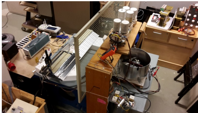
Figure 4.26: The whole setup: in the lower left corner is a wooden box containing transformers and rectifiers with a parallelly connected capacitor to give a stable DC input. On the top shelf is the set of capacitors which have the task of making the ringings sharper and on the leftmost bench is the prototype road.
