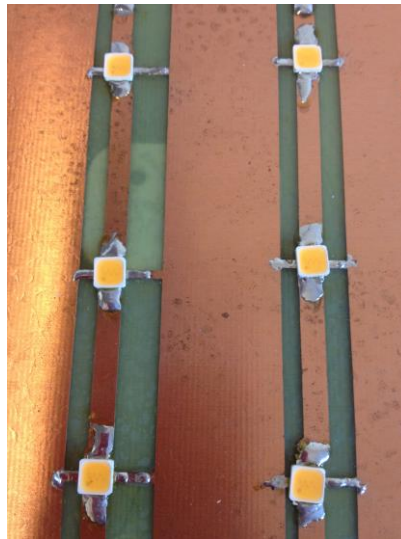
Fig. 51. The vertical LED lines with cooling pads between.
