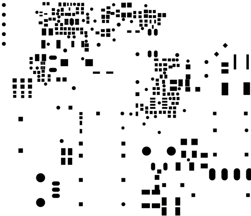
Fig. 26. A Gerber file containing information about where pads are located on our PCB design.
