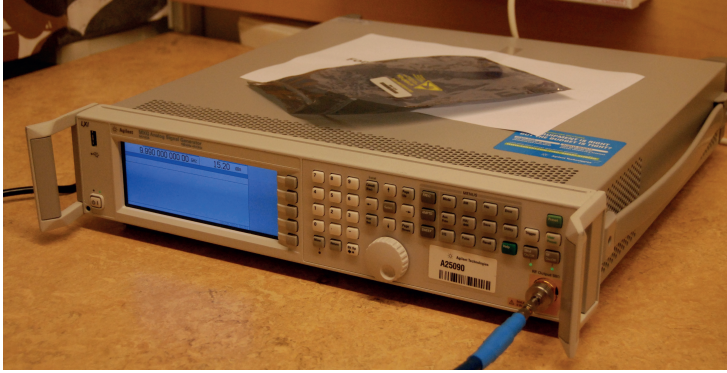
Figure 4.17: N5183A MXG microwave analog signal generator.
