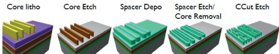
Figure 8: Manufacturing Process of SADP PROCESS (IMEC Process)
