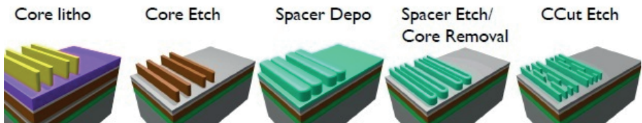
Figure 11. IMEC Fin Patterning Process
