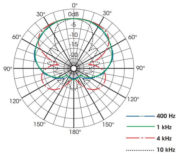
**Figure 3.4:** *Polar pattern of the external microphone*
