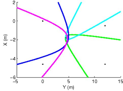
**Figure 2.4:** *The hyperbolas marked in different colors and microphone positions marked with black dots.*
