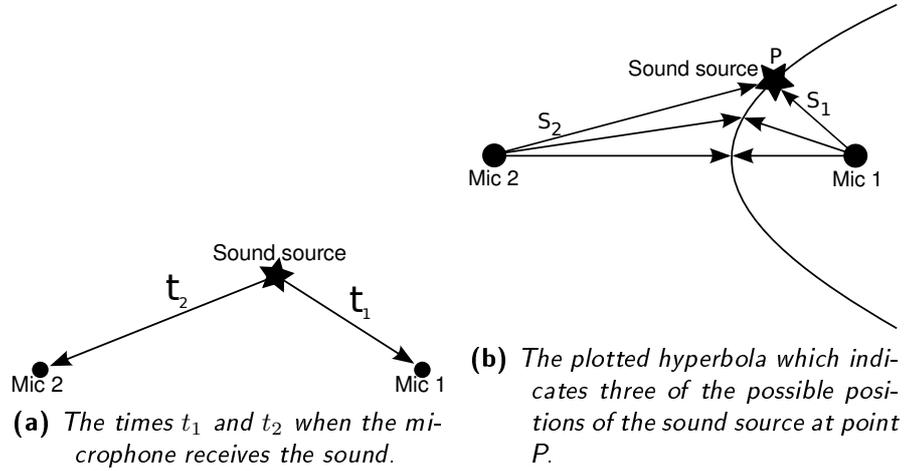
**Figure 2.3:** Positions of the sound source.
