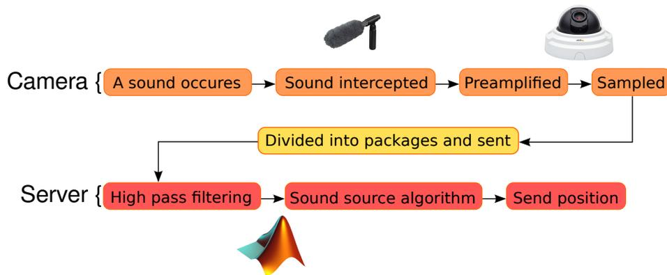
**Figure 3.7:** The summarized data flowchart of the system, showing how the data is being processed throughout the system.
