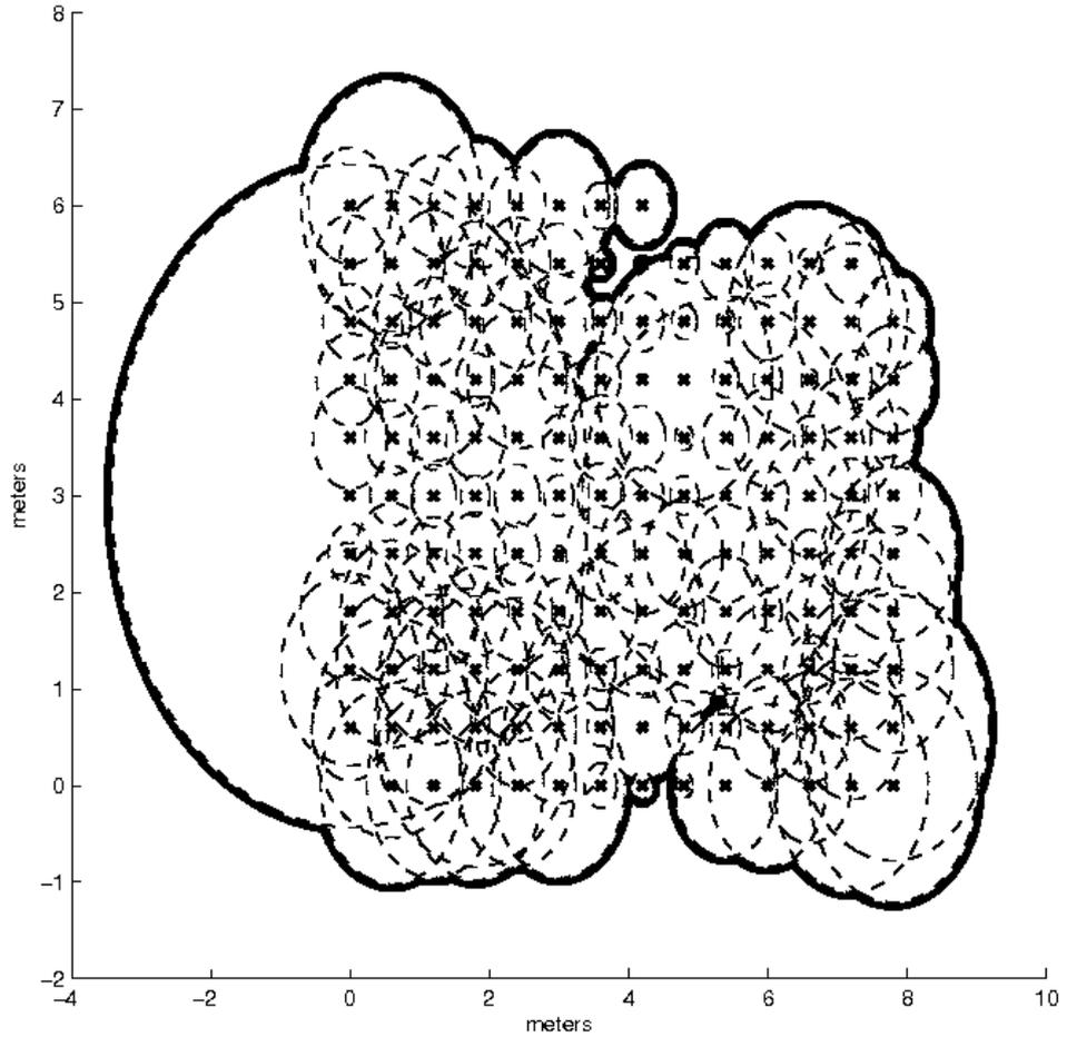
**Figure 4.4:** Plot showing where the sound (thump with stick) originated from along with their corresponding estimated error circle.
