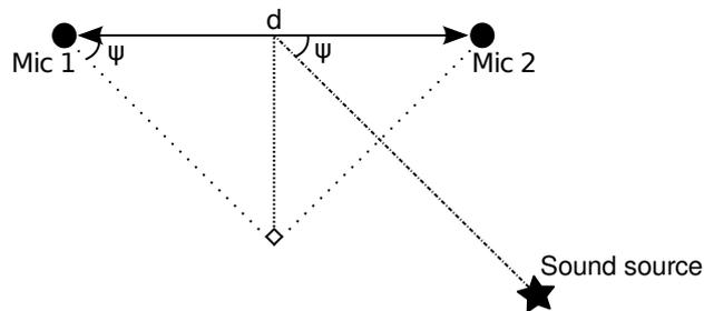
**Figure 2.1:** Using the triangulation to calculate from the direction of the sound source.
