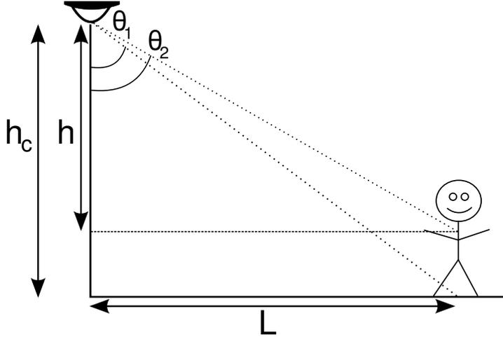
**Figure 2.5:** The PTZ camera pans and focuses itself on a elevated plane.  $h_c$  is the height of the camera,  $h$  is the distance to the elevated plane,  $\theta_1$  is the angle to the given position and  $\theta_2$  is the angle for the new position.
