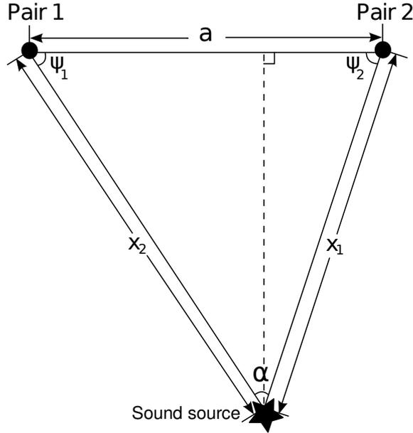
**Figure 2.2:** Determining the position of the sound source by using multiangulation. Each pair consists of two microphones.
