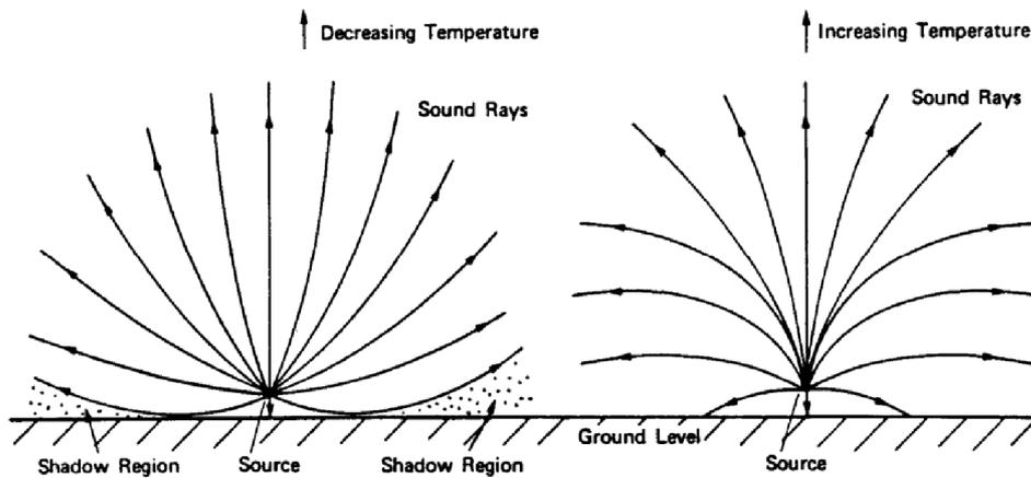
**Figure 2.6:** Impact on sound rays with decreasing and increasing temperature with increasing elevation.
