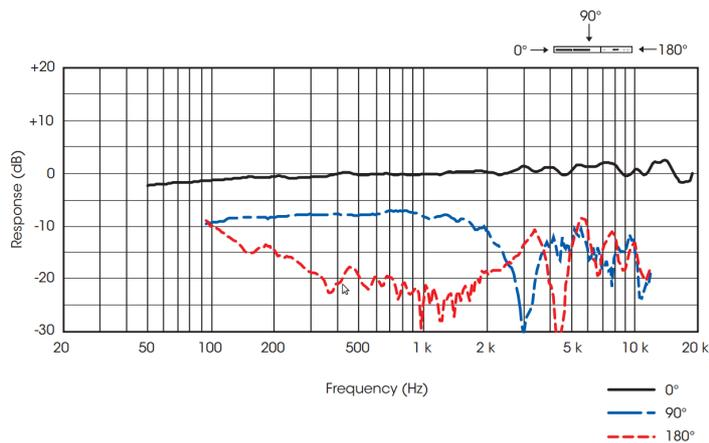
**Figure 3.5:** *Frequency response of the external microphone*
