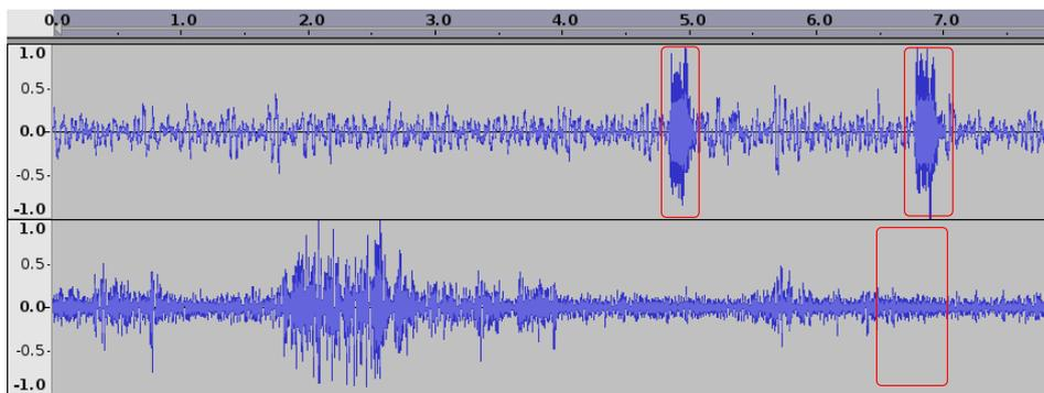
**Figure 3.1:** *Two different recordings done with the external microphone (top) and the internal microphone (bottom). The red frame marks the sound from the car horn.*
