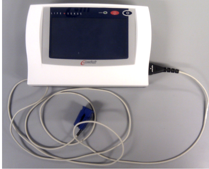
Figure 5.1: A Nonin Medair Life Sense PPG sensor.
