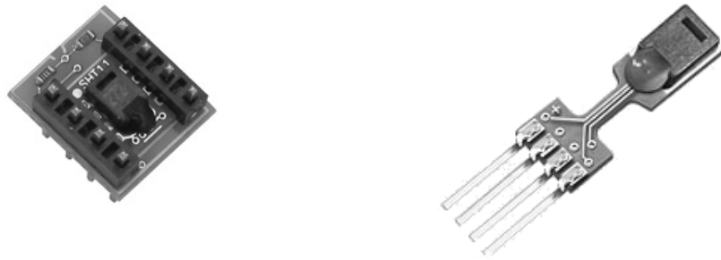
Figure 3.2: Left: SHT11 package mounted on breakout board. Right: SHT71 package.
