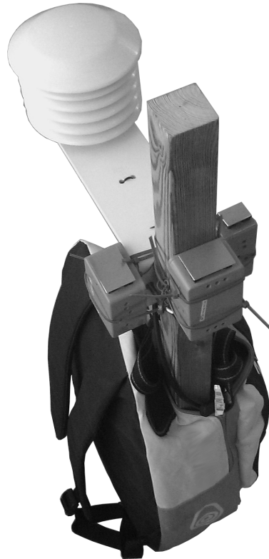
Figure 5.1: Measurement setup used outdoors consisting of the CS215 probe (Not visible due to radiation shield), logger, and the three sensor units.
