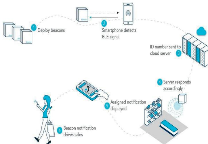
**Figure 2.1:** Basic working of BLE beacon [11]
