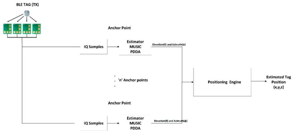
Figure 3.5: Position estimation flow using BLE technology [26].
