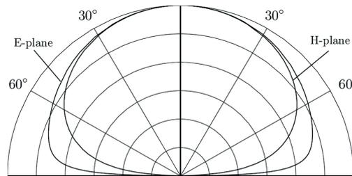
Figure 3.4: Radiation pattern of a Patch antenna [30]
