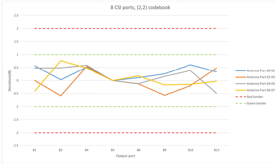
Figure 6.4: For each output port, the deviation between the simulation result and the measurement result, 8 CSI ports, (2,2) codebook
