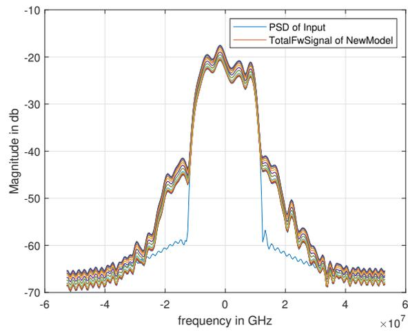
**Figure 4.25:** PSD of a load sensitive PA model
