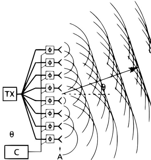
Figure 2.3: Antenna array radiation pattern [14]
