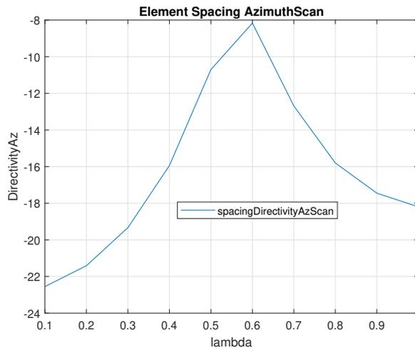
**Figure 4.12:** Embedded spacing scan of embedded URA
