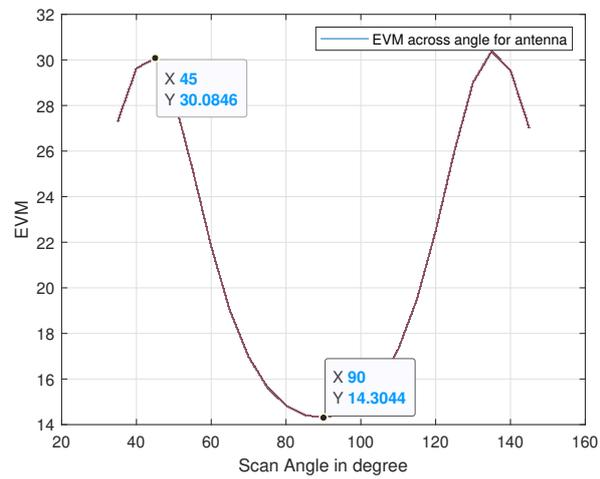
**Figure 4.23:** EVM for load sensitive PA model
