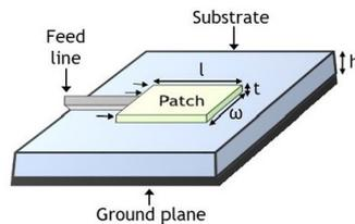
**Figure 3.2:** Patch Element Design [22]
