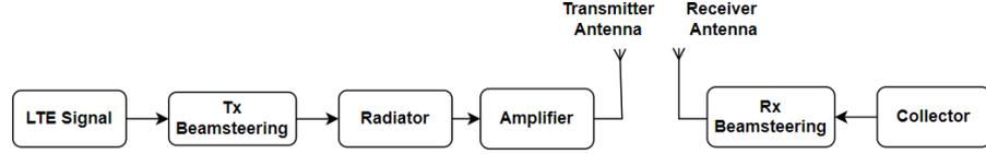
**Figure 3.8:** Block diagram of Tx Rx blocks
