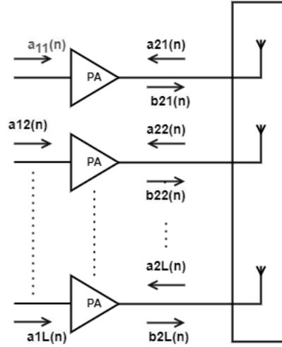
**Figure 3.9:** Multi-antenna Tx system [23]
