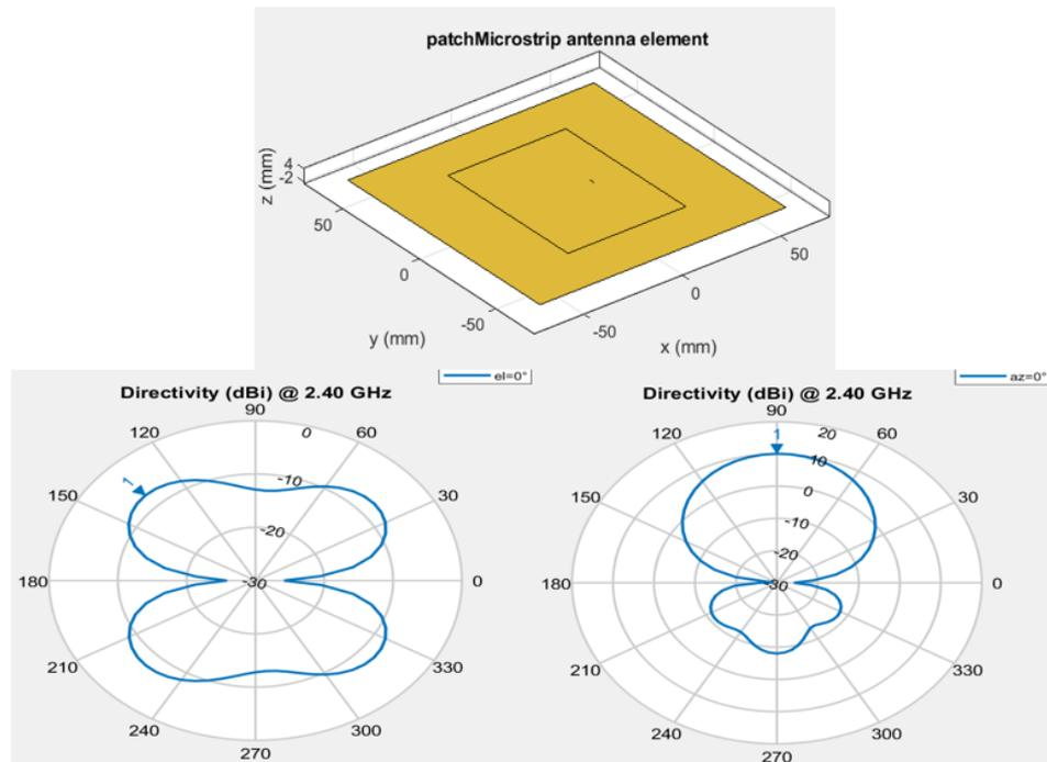
**Figure 3.3:** Patch element design, Az and El
