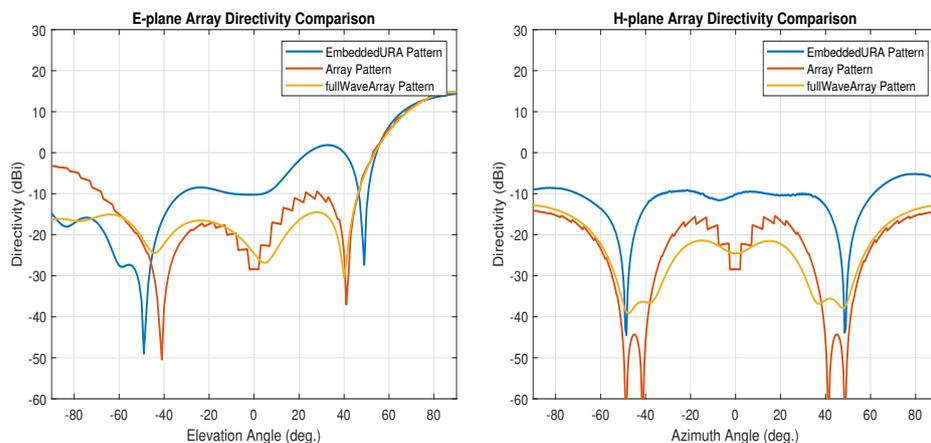
**Figure 4.10:** Embedded EI pattern comparison with full wave
