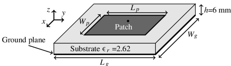
**Figure 2.1:** Patch Antenna Element in MATLAB [10]
