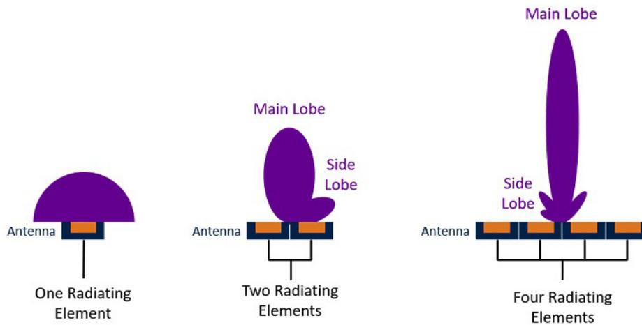
**Figure 2.2:** single and multi antenna array radiation pattern [13]
