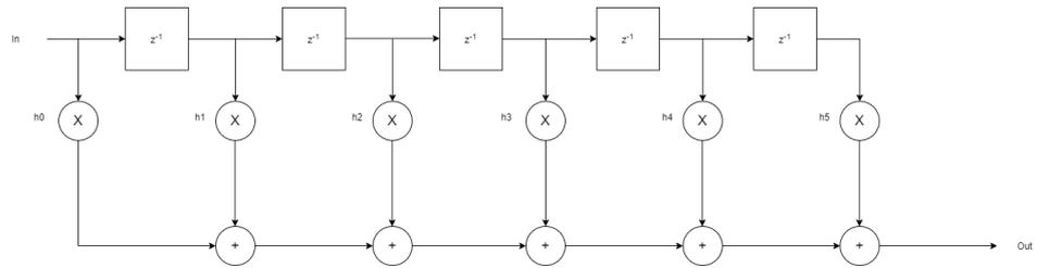
**Figure 3.1:** Block diagram of a direct form FIR
