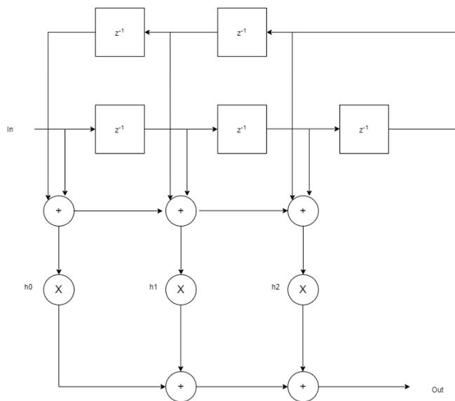
**Figure 3.2:** Block diagram of a symmetric FIR
