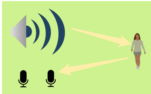
Figure 0.1: Motion detection at audio frequencies using speaker and microphone
