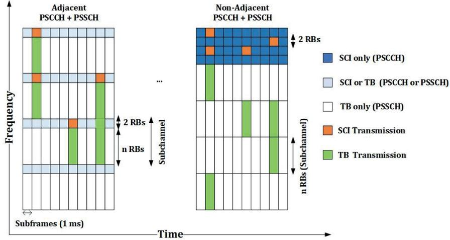
Fig. 3. LTE-V Subchannelization
