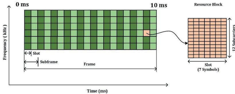
Fig. 2. LTE frame (1.4 MHz, Normal Cyclic Prefix)
