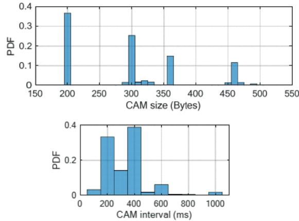
Fig. 5. CAM Sizes and CAM Intervals [15]
