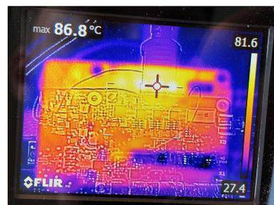
**Figure 7.11:** Thermal Image of the RX LNAs
