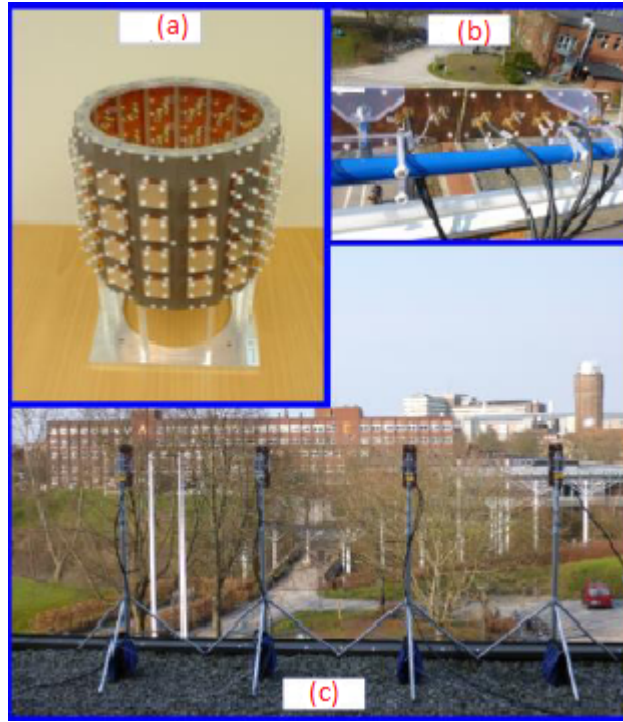
Figure 3.1: Antennas at the receiver and at the BS. (a) receiver antenna: stacked uniform cylindrical array with 64 cross-polarized antenna elements arranged in four rings. (b) BS antennas: co-located arrangement used in setup-II with inter-patch spacing of \lambda/2 (back view). (c) BS antennas: mounted on a tripod to facilitate adjusting the inter-patch spacing for setup-I, the photo is with inter-patch spacing of 1 m (back view).
