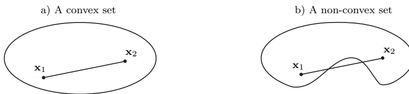
Figure 2: Illustration of a) A convex set in \mathbb{R}^2 . b) A non-convex set in \mathbb{R}^2 .
