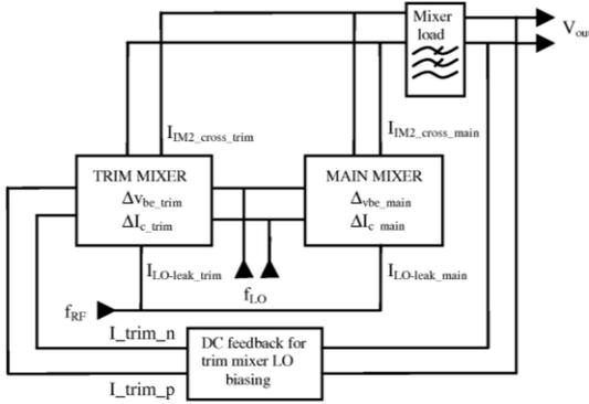
**Fig.3. Block diagram of the single ended mixer with IM<sub>2</sub>-suppression**
