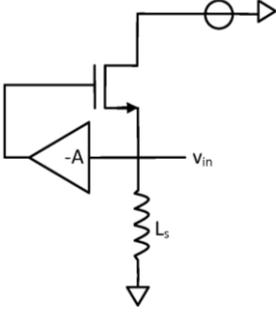
**Fig. 16. Common-gate LNA with  $g_m$ -boosting feedback**
