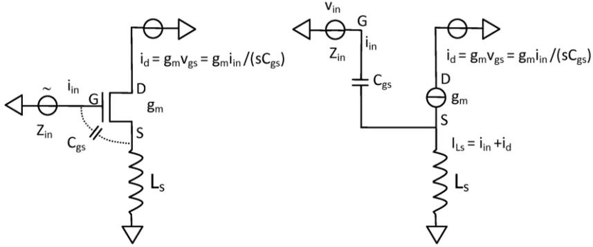
**Fig. 11. Architecture of the CS LNA with inductive degeneration**
