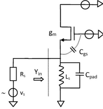
**Fig. 15. Architecture of the CG LNA including parasitics**
