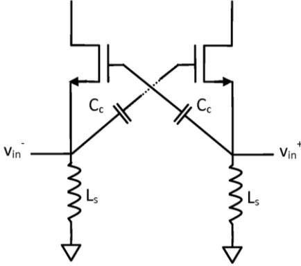
**Fig. 17. Differential CG LNA with capacitive cross coupling**
