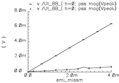
**Fig.9. Differential DC-offset in mV at mixer I output versus V<sub>be</sub> mismatch with and without feedback**
