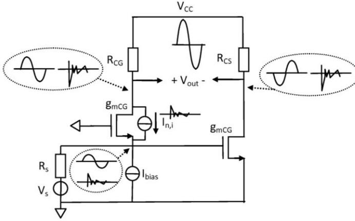
**Fig. 22. Noise cancellation with combination of CS- and CG stage**
