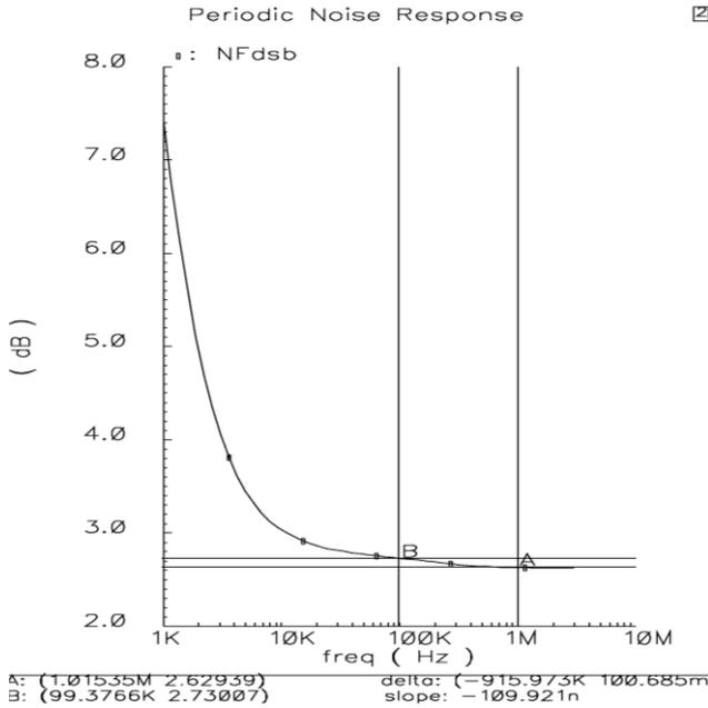
**Fig.12. Band I noise figure in AC-coupled mode**
