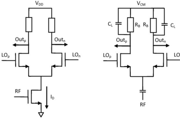
Fig. 26. Single ended active and passive mixers
