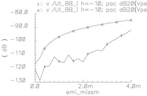
**Fig.8. Differential IM<sub>2</sub> level in dBVp at mixer I output versus V<sub>be</sub> mismatch with and without feedback**
