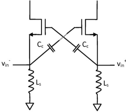
**Fig. 17. Differential CG LNA with capacitive cross coupling**
