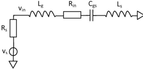
**Fig. 12. Model for input matching Q-value calculation**
