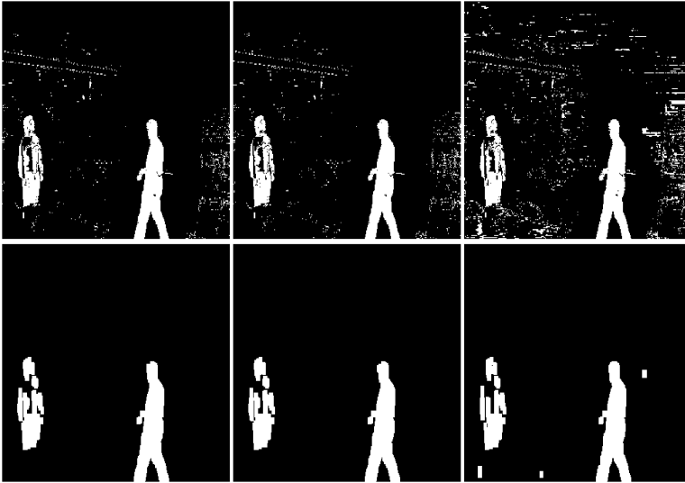
Figure 1.25: The results before and after morphological filtering for different thresholds: (left) Original result, (middle) Threshold of 0.8, (right) Threshold of 0.4.
