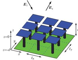
High-impedance surfaces are often composed by periodic structures above a PEC ground plane, here a mushroom structure.
