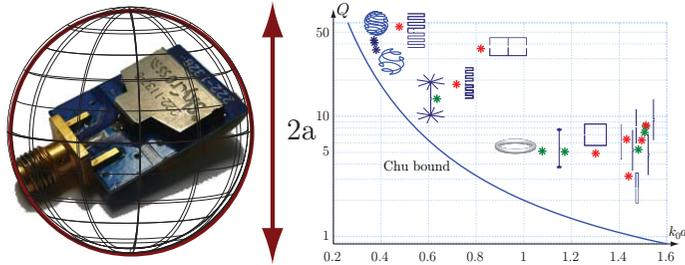
Calculation of the stored energy and radiated power outside a sphere with radius  $a$  gives the Chu-bounds (1948) for omni-directional antennas, *i.e.*,
