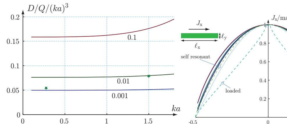
The stars indicate the performance of strip dipoles with  $\xi = 0.01$ . Almost no dependence on  $ka$  for  $D/(Qk^3 a^3)$ . More dependence on  $ka$  for  $D$  and  $Qk^3 a^3$ . Note the directivity of the half-wave dipole.
