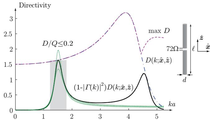
Lossless  $\hat{z}$ -directed dipole, wire diameter  $d = \ell/1000$ , matched to  $72\Omega$ . Weighted area under the black curve (partial realized gain) is known. Note, half wavelength dipole for  $ka = \pi/2 \approx 1.5$  with directivity  $D \approx 1.64 \approx 2.15$  dB<sub>i</sub>.
