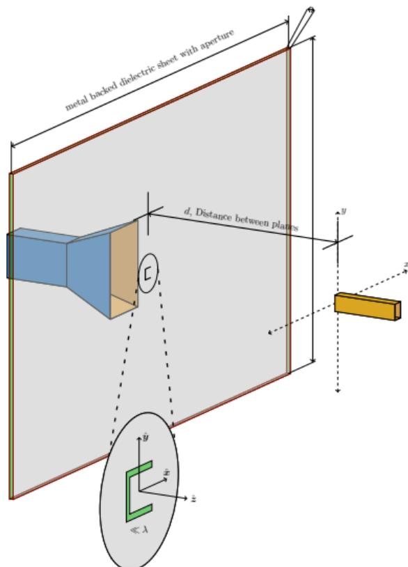
**Aperture Sheet:** Aperture cut out from metal backed dielectric.
