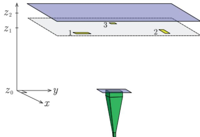
The received field and the field at the imaging plane are dominated by the illuminating field. Not sparse in a pixel basis and hence not suitable for CS.
