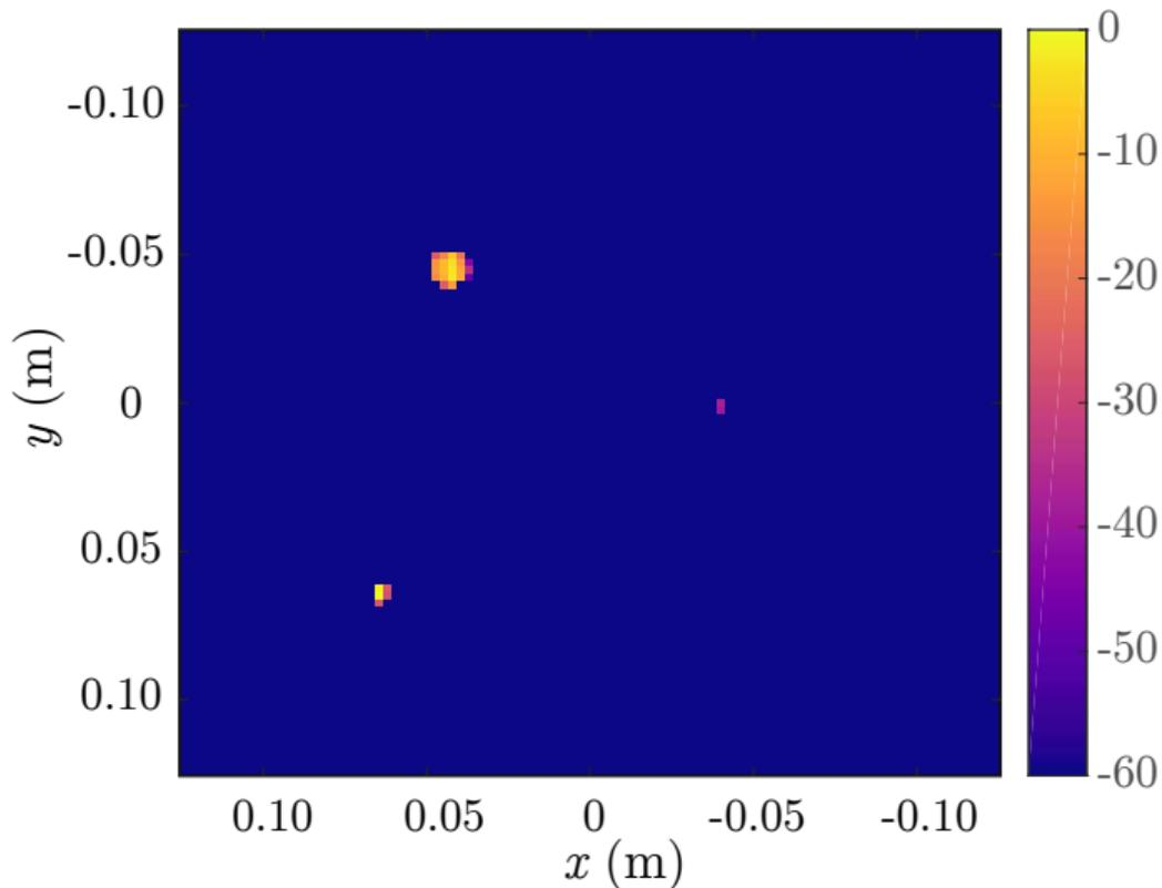
Compressive sensing with source separation. 60 dB range
