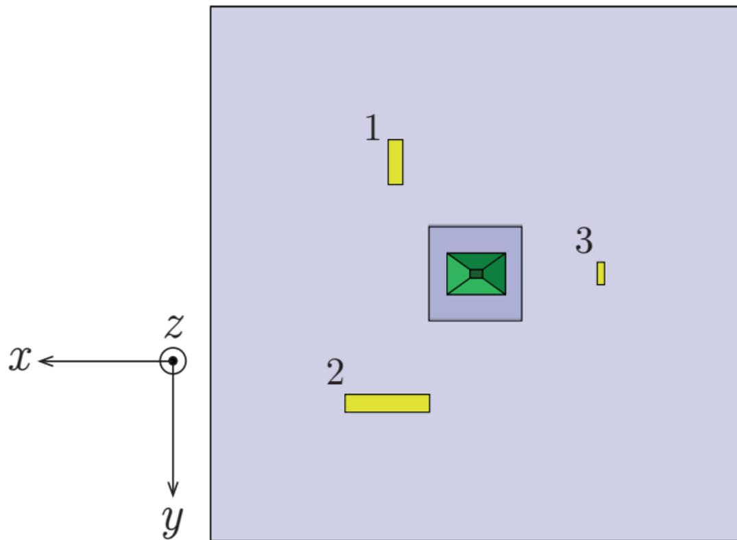
Simulation (FEKO) setup with 3 defects: top view
