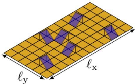
Consider a planar rectangle divided into  $N_x \times N_y$  elements with a current density  $\mathbf{J}(\mathbf{r})$  expanded in local basis functions  $\psi_m(\mathbf{r})$
