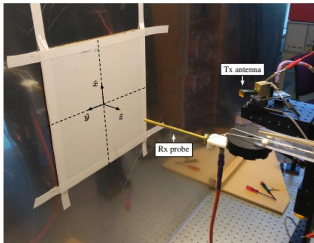
Mount the DUT on top of a ground plane to emulate/extend the underlying conducting layer
