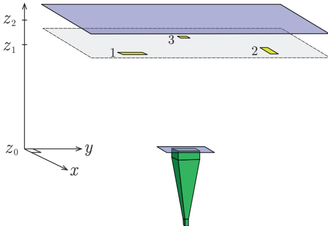
Simulation (FEKO) setup with 3 defects: side view
