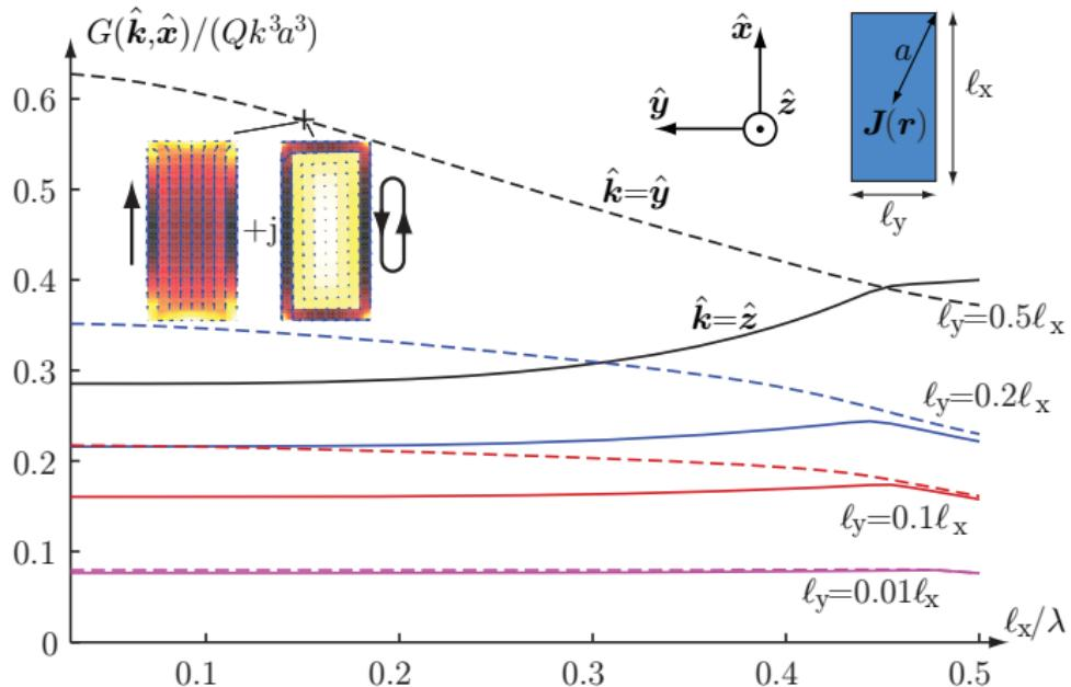
Solution for current densities confined to planar rectangles with side lengths  $\ell_x$  and  $\ell_y = \{0.01, 0.1, 0.2, 0.5\}\ell_x$ .
