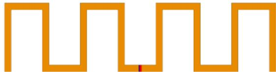
Antenna geometry with feed point.
