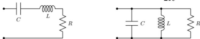
**Small open-circuit antennas** Model based on the (small) electrical dipole, cf., the Chu bound (1948)
