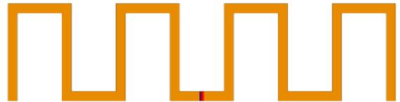
Antenna geometry with feed point.
