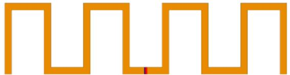
Antenna geometry with feed point.
