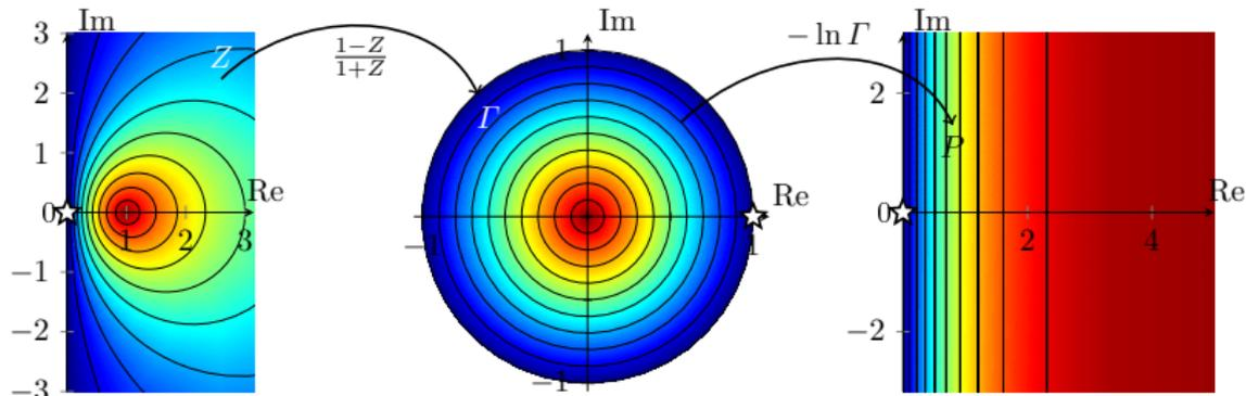
The absorber is an example with scattering parameters  $|\Gamma(0)| = 1$  where it is desired to have  $|\Gamma(\omega)| \leq \Gamma_0$ .
