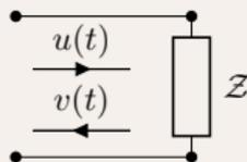
Passivity is a systems concept. Not sufficient with passive materials (devices). Need less energy in the output signal than in the input signal for all times and signals.
