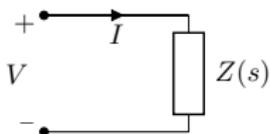
**Example:** Reflection coefficient  $H(s) = \Gamma(s) = \frac{Z(s) - Z_0}{Z(s) + Z_0}$ ,  $V = \Gamma U$ .
