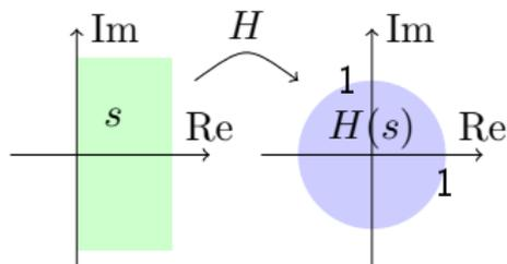
**Example:** Impedance  $H(s) = Z(s)$  of a passive circuit,  $V = ZI$ .
