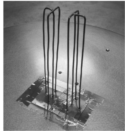
Best, *et al.*, An Impedance-Matched 2-Element Superdirective Array, IEEE-TAP, 2008
