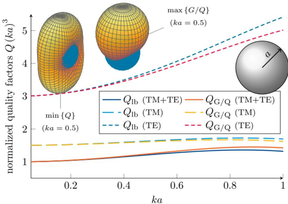
$Q_{lb}$  and Q-factors from  $G/Q$  are similar. Degenerate eigenvalues (symmetries)  $Q_{lb}$  same for the Huygens source ( $G/Q$ ) as for the equiphase current.
