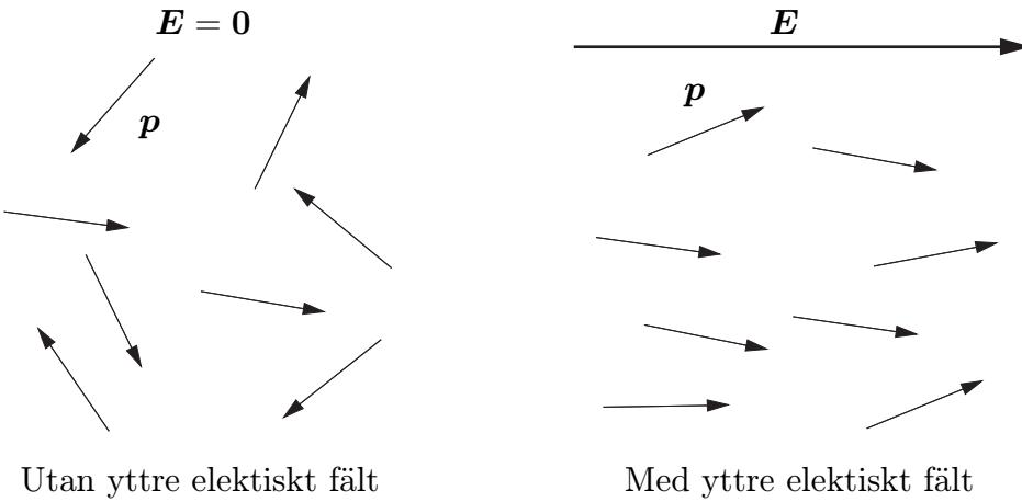
**Figur 1.6:** Permanent polarized molecules with or without external electric field.
