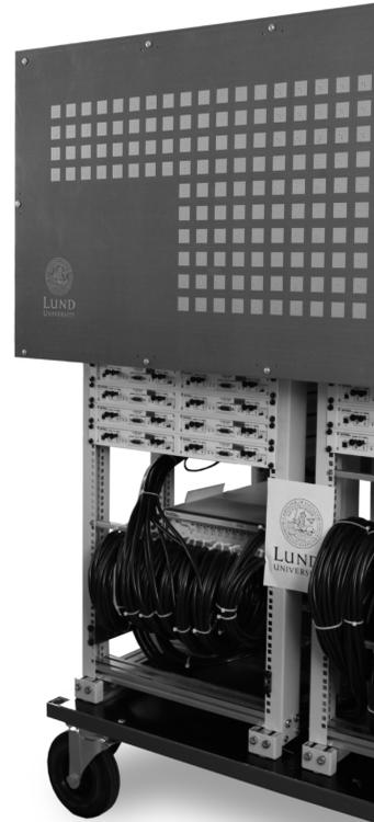
**IMAGE »** The Lund University massive MIMO testbed, LuMaMi, with all its antenna elements at the front and the radio units behind. The testbed, including the antenna, is 1.2 m wide and 1.5 m tall.
