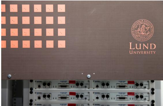
**IMAGE »** Part of the Lund University massive MIMO testbed, LuMa-Mi, with 20 of the 100 antenna elements at the front and some of the radio units behind.
