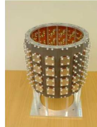
128-port cylindrical antenna array
