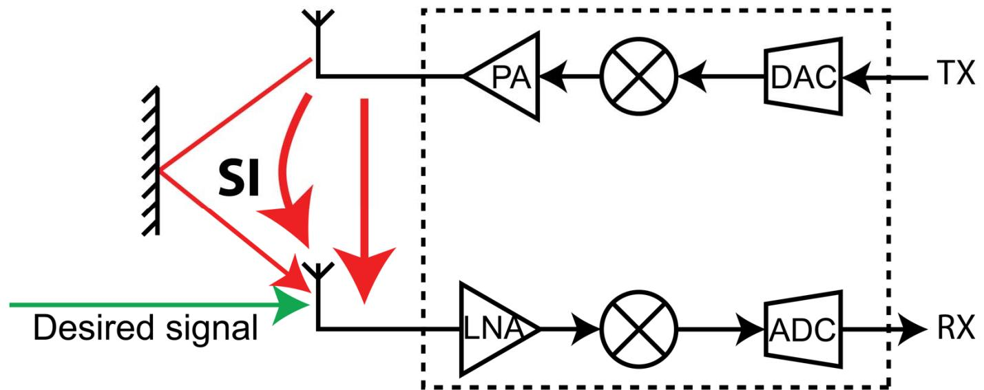
Handheld device → varying antenna isolation
