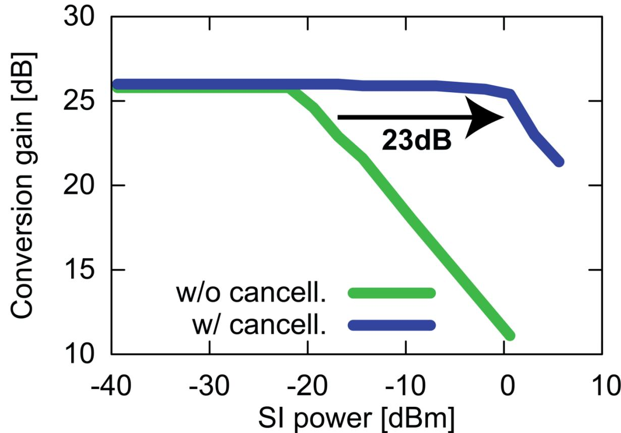
Desired signal only compressed at  $> 0$  dBm SI
