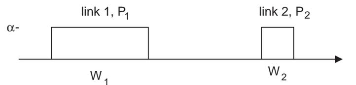
The average received signal power used in link 1 is  $P_1$  (and  $P_2$  in link 2). Hence, the capacity of link 1 is  $C_1 = W_1 \log_2 \left( 1 + \frac{P_1}{N_0 W_1} \right)$  (and  $C_2$  in link 2).
