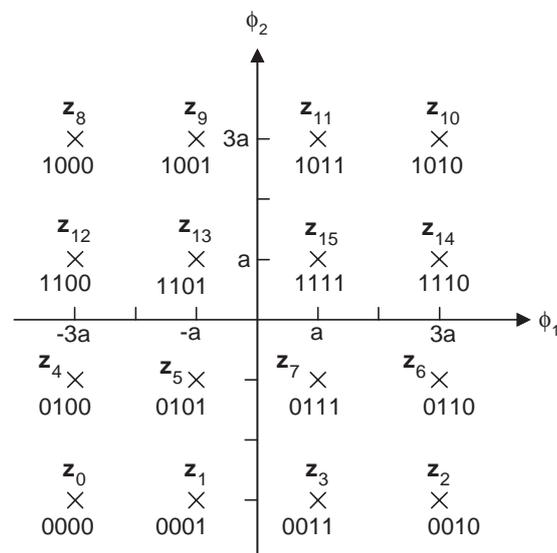
a) Assume that the four bits 1101 are sent, and that the correlator output  $\mathbf{r}$  in the receiver is
