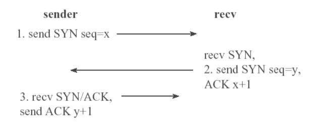
both sides can SYN at the same time and it will work results include established connection, initial sequence numbers exchanged, ACKS ack next expected byte (cumulative)
