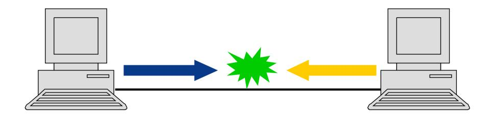
If two devices transmit simultaneously, the signals will be mixed and destroyed.
