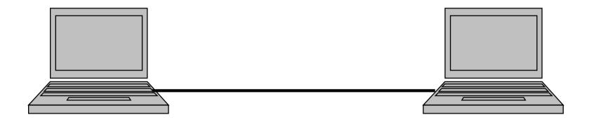
Two devices communicate over a *link*. The link uses some form of *medium*.
