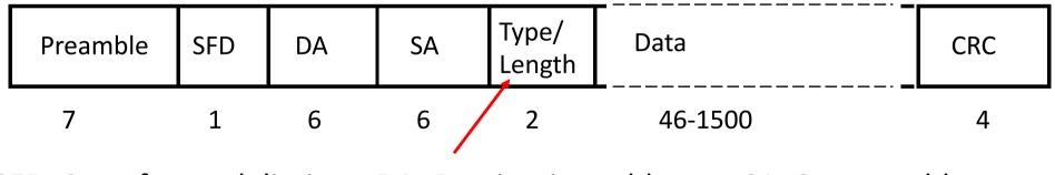
SFD=Start frame delimiter DA=Destination address SA=Source address
