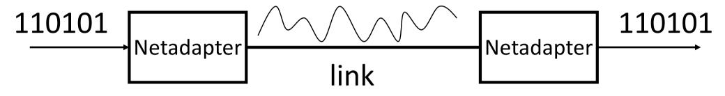
The transmitter has a network adapter that transforms the bits into signals, which are transmitted over the link.
