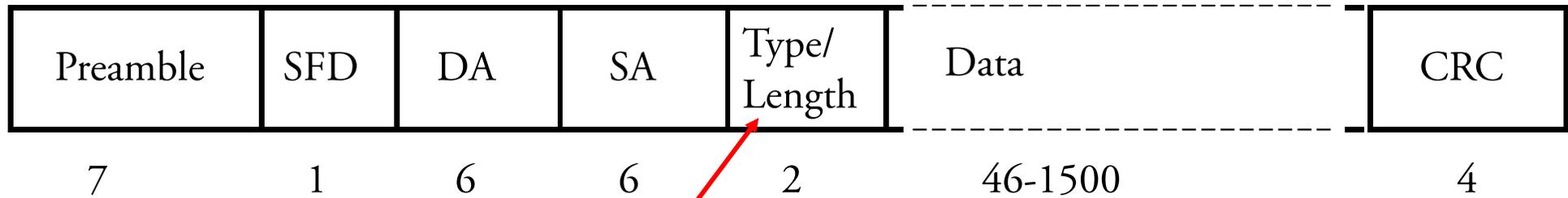
SFD=Start frame delimiter    DA=Destination address    SA=Source address
