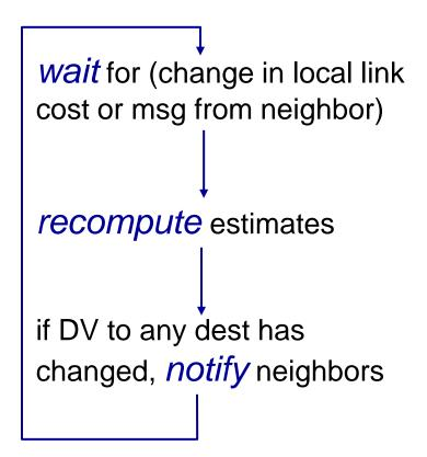
$$D_{x}(y) = min\{c(x,y) + D_{y}(y), c(x,z) + D_{z}(y)\}$$
