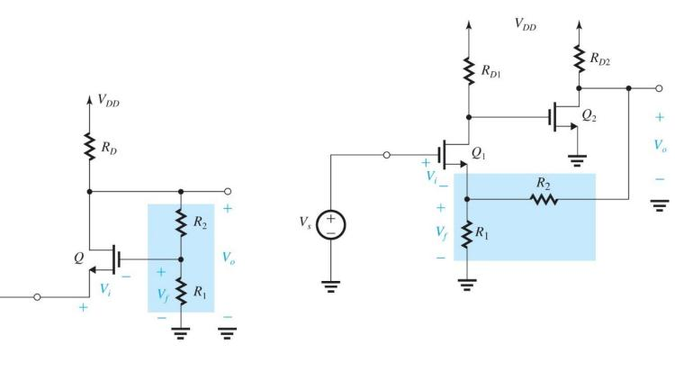
The feedback network is treated as an add-on to the amplifier.
