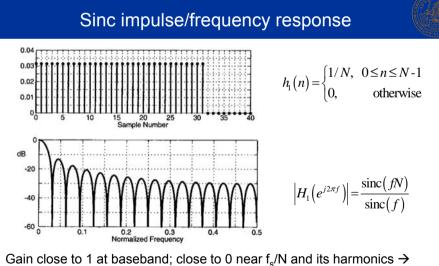
Gain close to 1 at baseband; close to 0 near  $f_s/N$  and its harmonics  $\neg$ if the sampling rate at the output is reduced by N, causing the noise around  $f_s/N$ ,  $2f_s/N$ , ..., to fold into the baseband, the energy of the aliased noise will be reduced by the attenuation of the sinc filter  $\rightarrow$ N=OSR should be chosen
