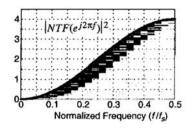
Quantizer error from internal ADC is white  $\rightarrow$  its power is  $\Delta^2/12 = 1/3$ , and its power is found between DC and Nyquist =  $f_s/2$  (=0.5 normalized to the sampling frequency)  $\rightarrow$  thus, the spectral power density is
