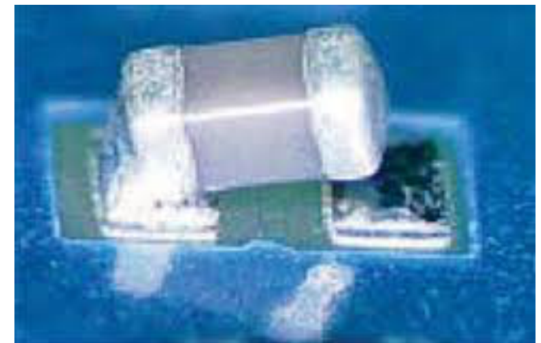
Fig. 1. With "tombstoning" only one side of a two-leaded chip component may be soldered to the target pad, but its other termination may not come in contact with the associated target pad. Photo courtesy of IPC 630
