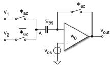
Two-phase approach  $\rightarrow$  during  $\Phi_{az}$ , opamp in unity-gain configuration  $\rightarrow C_{os}$  is charged to  $V_{os}$ - $V_1$ ; during the second phase, we have
