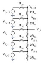
Besides this, interpolating resistors + pre-amps with finite output resistance average the offsets of the pre-amps, improving the overall linearity The current flowing into the i-th pre-amp is
