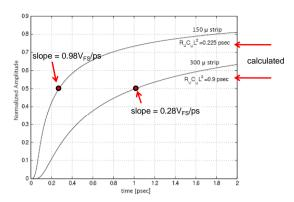
A noise of  $40\,\text{mV}_{FS}$  in the crossing threshold (0.5 normalized amplitude) results in a jitter of 40.8fs and 142.8fs, respectively; e.g.
