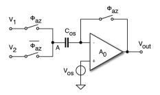
One terminal is the input of the flash, the other is the tap from the ladder → the difference between input and reference is not calculated by a differential pair, but by the previous voltage subtraction at node A!
