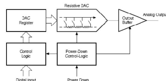
The decoding method used to select the divider voltage depends on a trade-off between speed, complexity, and power consumption
