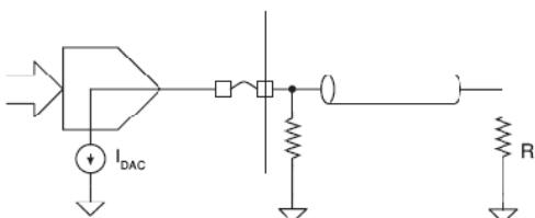
Often a current is used to drive an off-chip coaxial cable to yield a voltage across the terminations
