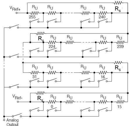
$R_S$  in parallel to  $k R_U$  units: higher speed, but also higher power consumption; for each line, the equivalent resistance is
