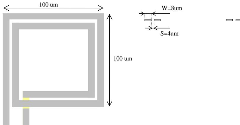
Assume there are no Eddy current losses in the substrate, and no proximity effect in the metal track.
