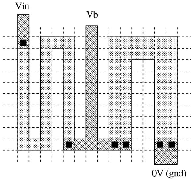
The terminal  $V_b$  is unloaded, that is no current flows in or out of the  $V_b$  terminal.
