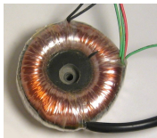
Transformator ( \sim 1 \text{ T} )
