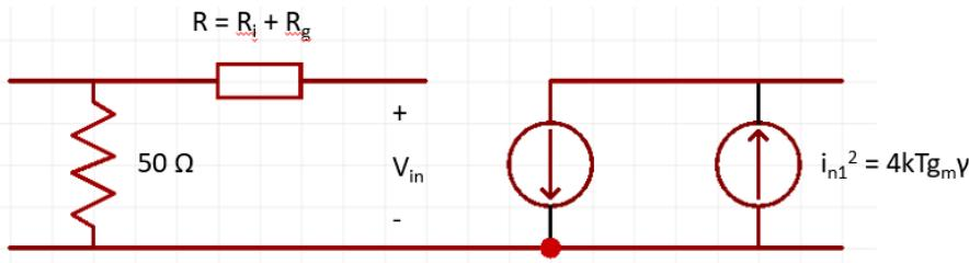
$i_{n1}^2$  represent the noise due to drift/diffusion in the FET
