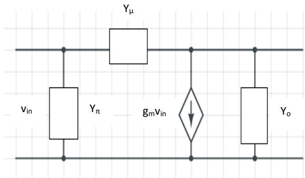
The hybrid parameters are,  $Y_\pi = Y_{11} + Y_{12} = \frac{1}{\left( 8R + \frac{3}{j\omega C} \right)}$
