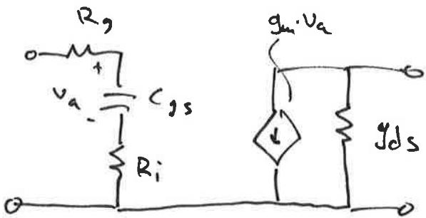
$$R_i = \frac{1}{i_g \cdot g_m} \quad : \text{Set } R_i + R_g = R$$
