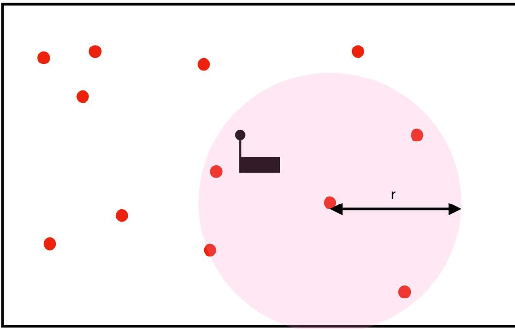
The sensors operate in a cyclic manner where they sleep during an interval and then wake up to send a measurement report to the gateway. The time it takes to send the message is  $T_p$  s and we deem the propagation time negligible (it takes no time for the message to reach the gateway). The sleep interval is exponentially distributed with mean  $t_s$ .
