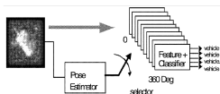
Fig. 4. Classifier topology is depicted. First a pose estimator is applied to image and determines approximate pose of target, then classifier is chosen according to result of pose estimation.
